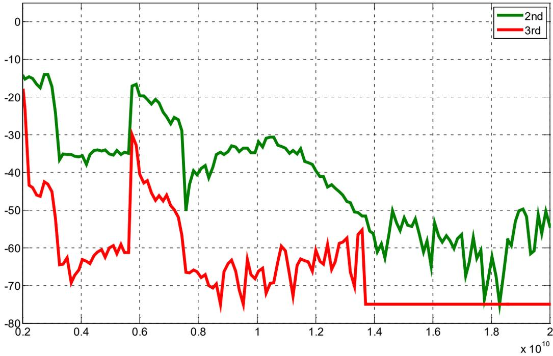
Harmonic output power [dBc] vs. frequency [Hz]
